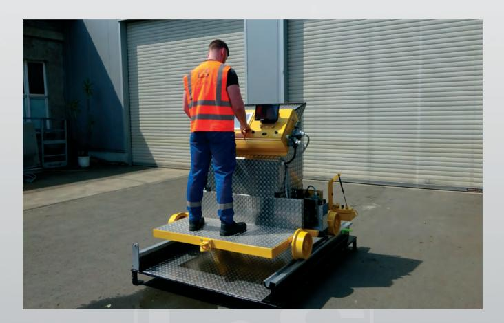
The TMD 2-4 is an efficient solution for the detection of transverse profile on left and right rail of tracks. The online measuring device TMD 2-4 is applicable for grooved rails and standard Vignol rails.
