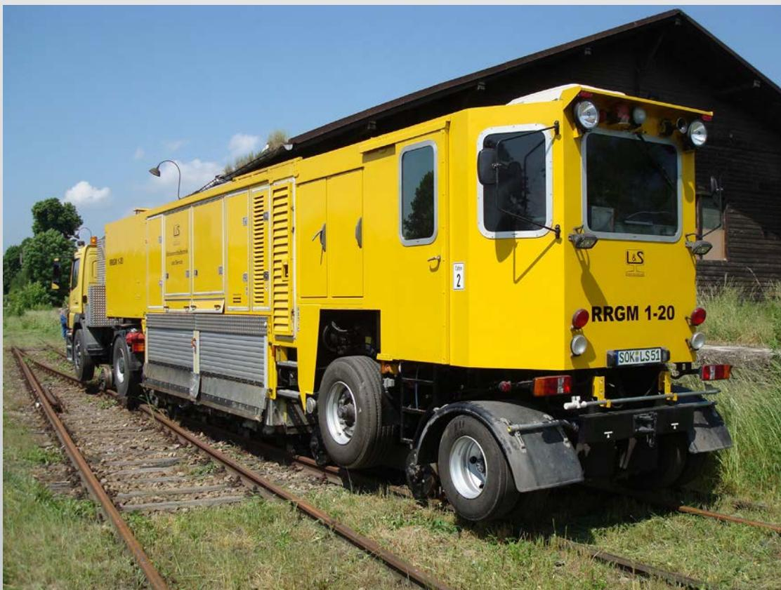
The rail grinder RRGM 1-20 is a rail-road going machine. The machine has 20 grinding spindles with independent angular adjustment. They are driven by 7,5 to 15 kW frequency-controlled electrical motors. The computer monitored grinding process is controlled with touch pad by the operator inside of the cabin.
