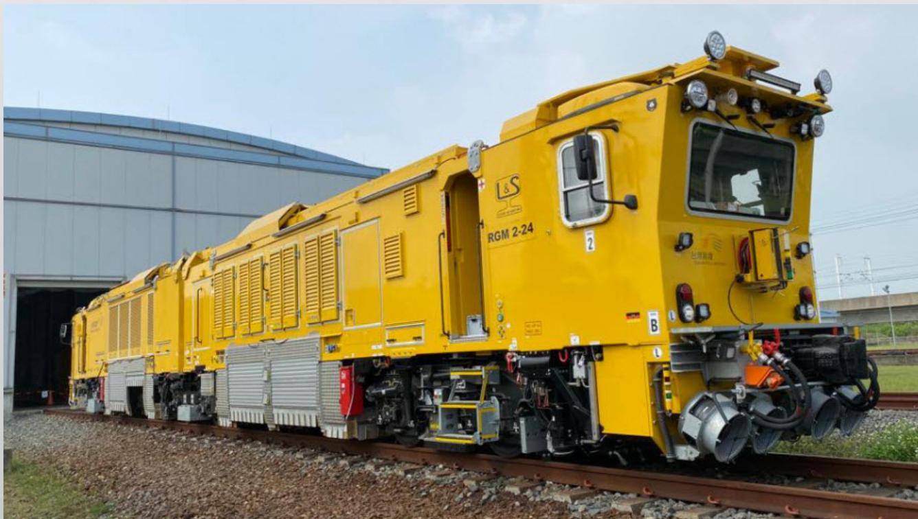
The rail grinder RGM 2-24 is a rail-borne machine which is consisted of two wagons and has 24 grinding spindles with independant angular adjustment. Each of the spindles is driven by a frequency-controlled electrical motor. The computer monitored grinding process is controlled with touch pad by the operator inside of the cabin.
