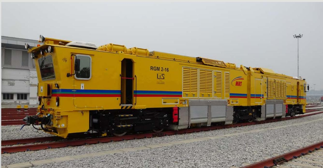
The rail grinder RGM 2-16 is a rail-borne machine which is consisted of two wagons and has 16 grinding spindles with independant angular adjustment. Each of the spindles is driven by a frequency-controlled electrical motor. The computer monitored grinding process is controlled with touch pad by the operator inside of the cabin.
