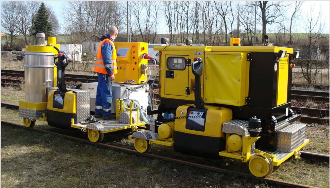
The LRGM 1-2/ AM16 is a turnout grinding machine for the machining of the rail head which composes except the grinding unit also a generator so that no power cables has to be installed along the working site. The grinder can be easily railed in and out with a ramp of a rail vehicle, by crane or by an assembled lifter with steering function.
