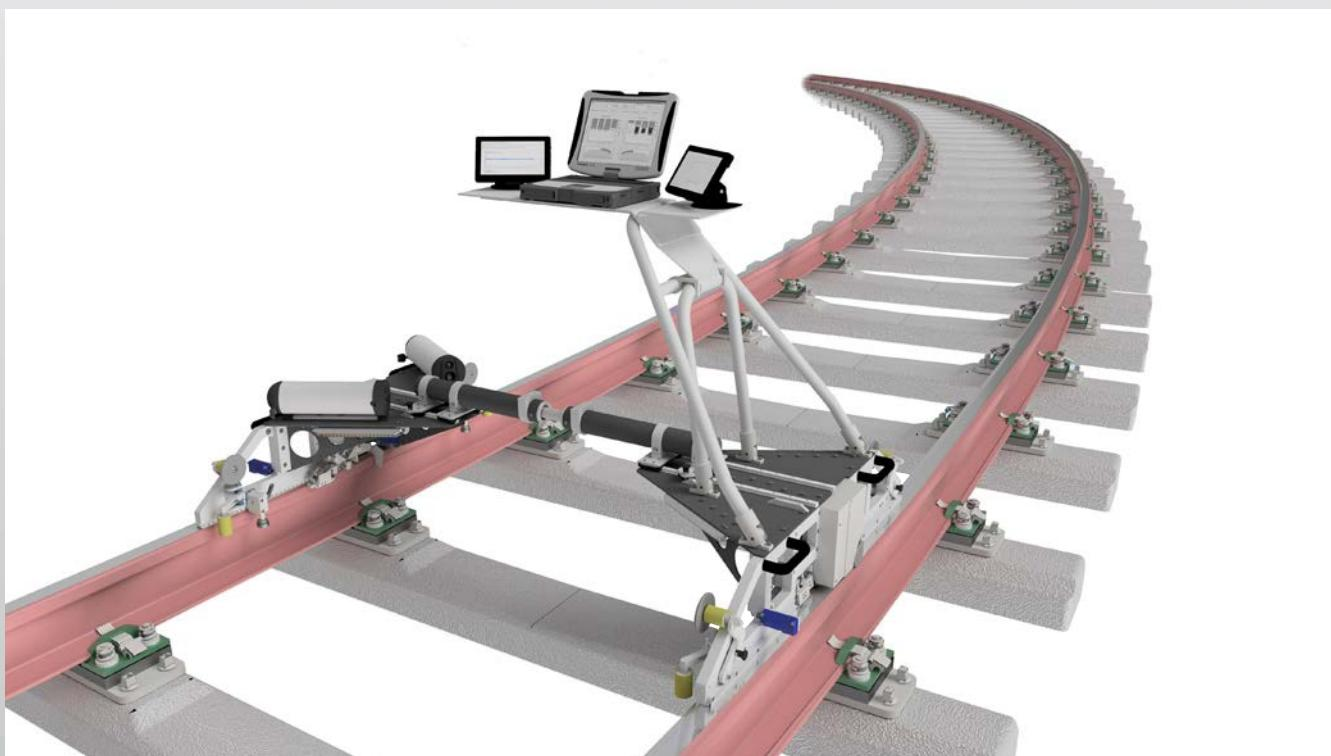
The LTMD 2-4-HC is an efficient solution for continuous measurement on tracks as well as for continuous or point measurement in switches. The online measuring device LTMD 2-4-HC can be used for grooved rails and standard Vignol rails in track systems with track gauges 900-1435 mm and enables simultaneous measurement of the left and right rails. The following measuring methods are integrated:
